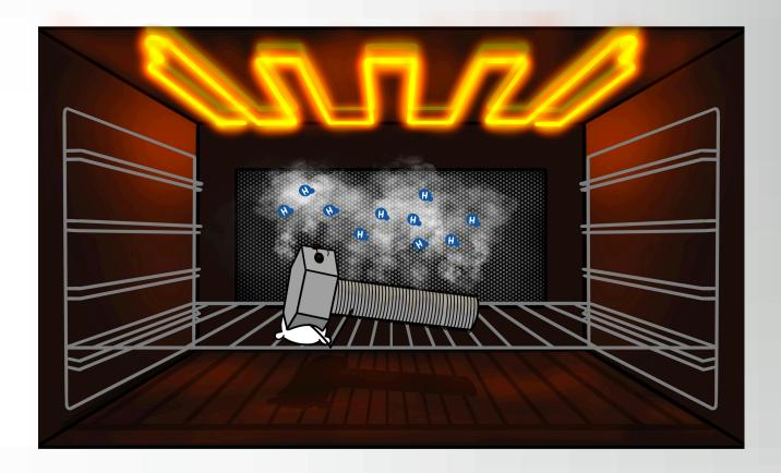
Baking is the other key to reducing embrittlement. Also known as "Low Hydrogen Annealing," it's commonly referred to as "baking" because the process involves heating fasteners in an oven for a prescribed amount of time. Heating newly plated fasteners and holding them at a certain heat for the correct amount of time allows the excess hydrogen atoms to escape the fastener's steel structure.
