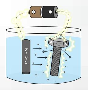
During the electroplating process, a fastener is hooked up to an electric current, which attracts the zinc ions in the plating solution to deposit in a thin layer over the fastener's surface. If this part was first subjected to acid pickling, the electric current and zinc coating seal the surface of the part, trapping the absorbed hydrogen inside.
