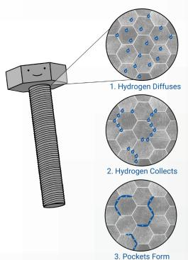
When pressure is applied to an embrittled fastener in assembly, the hydrogen atoms migrate to high-stress areas of the part, creating brittle chemical compounds and weakening those areas. Hydrogen Embrittlement fractures most commonly appear directly underneath the head and at the point where the shoulder meets the threads.
