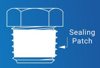
Sealing patches are applied a full 360° around the threads. On pipe and hydraulic fittings, the first one to two threads are left free of the patch material and then the remaining threads are coated. For screw threads the sealing patch is typically applied to the first five to ten threads of the screw.
