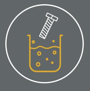
Coating refers to the use of powder or chemical additions to the surface of the fastener. This process involves dipping the item into a chemical bath, with the product then spun out at high speeds to remove any excess material. This dip and spin process will create the specified thickness of the coating.
