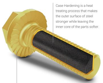
The case hardened surface adds strength and toughness to the serrations on a Hex Serrated Flange Screw providing resistance to rounding off and ensures that they bite into the surface they are being installed on.
